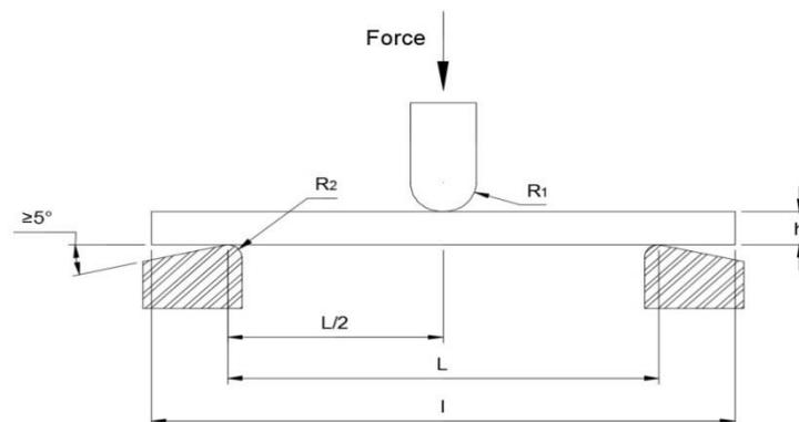
Length of specimen l = The specimen shall be long enough to allow for overhanging on each end of at least 10 % of the support span.
