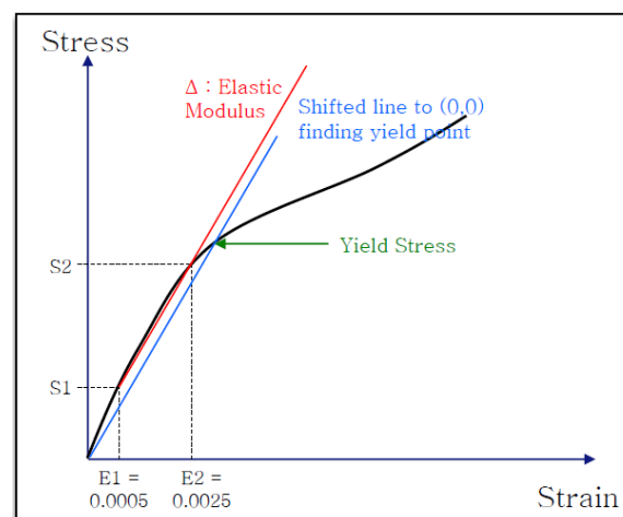
(Figure 1) Modulus and yield stress according to ISO
