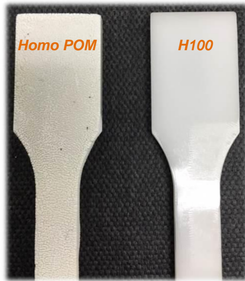
[Figure 6] Heat resistance (color change) of KEPITAL H100
