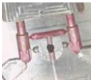
[Figure 2] Mold deposit by migration of pigments
