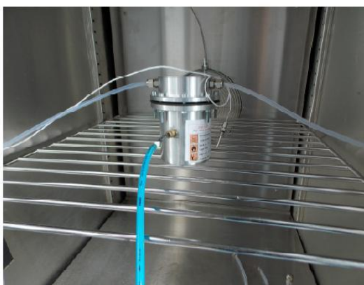
Sample inside Micro-SHED for emission test
