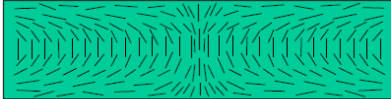
Figure 5. Fiber Orientation in Weld Line
